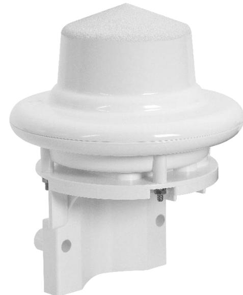
The Radar measurement principle offers extremely fast response time. Precipitation intensity can be detected up to 200 mm/h and drop of up to 5.0 mm can be recognized.
